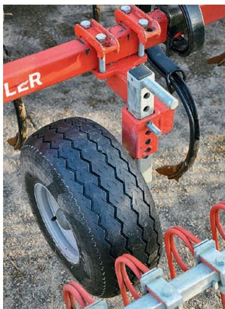
The optional 18.5x8.5-8 wheels at the rear keep the cultivator running level. Unfortunately, these only have manual adjustment.
