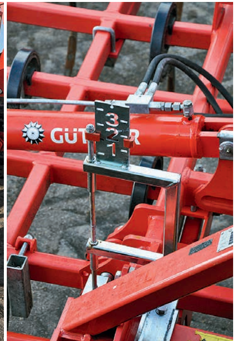
The four 185/65 R14 gauge wheels positioned out front give effective depth control. They are hydraulically adjusted, with a decent-sized scale making changes easy.
