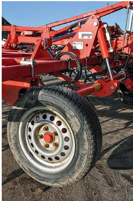
The four 185/65 R14 gauge wheels positioned out front give effective depth control. They are hydraulically adjusted, with a decent-sized scale making changes easy.
